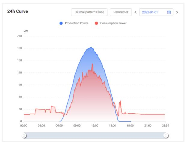
• **Data Overview**: The recent data changes of the power station are displayed through statistics of the power generation and power consumption data of the power station, so that users can more intuitively understand the summary and expected income of the power generation and power consumption of the photovoltaic power station, and support switching the data records of different dates [today] and [this
